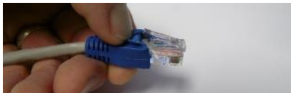
Pull boot back to access lock clip
