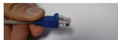
Slide boot back over lock clip
