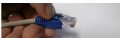
Pull boot back to access lock clip
